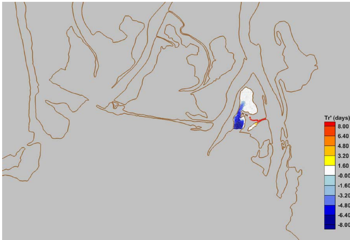
Figure 64. Predicted change in residence time (Tr') from Case 002 to Case 202 as a function of particle initial position.
