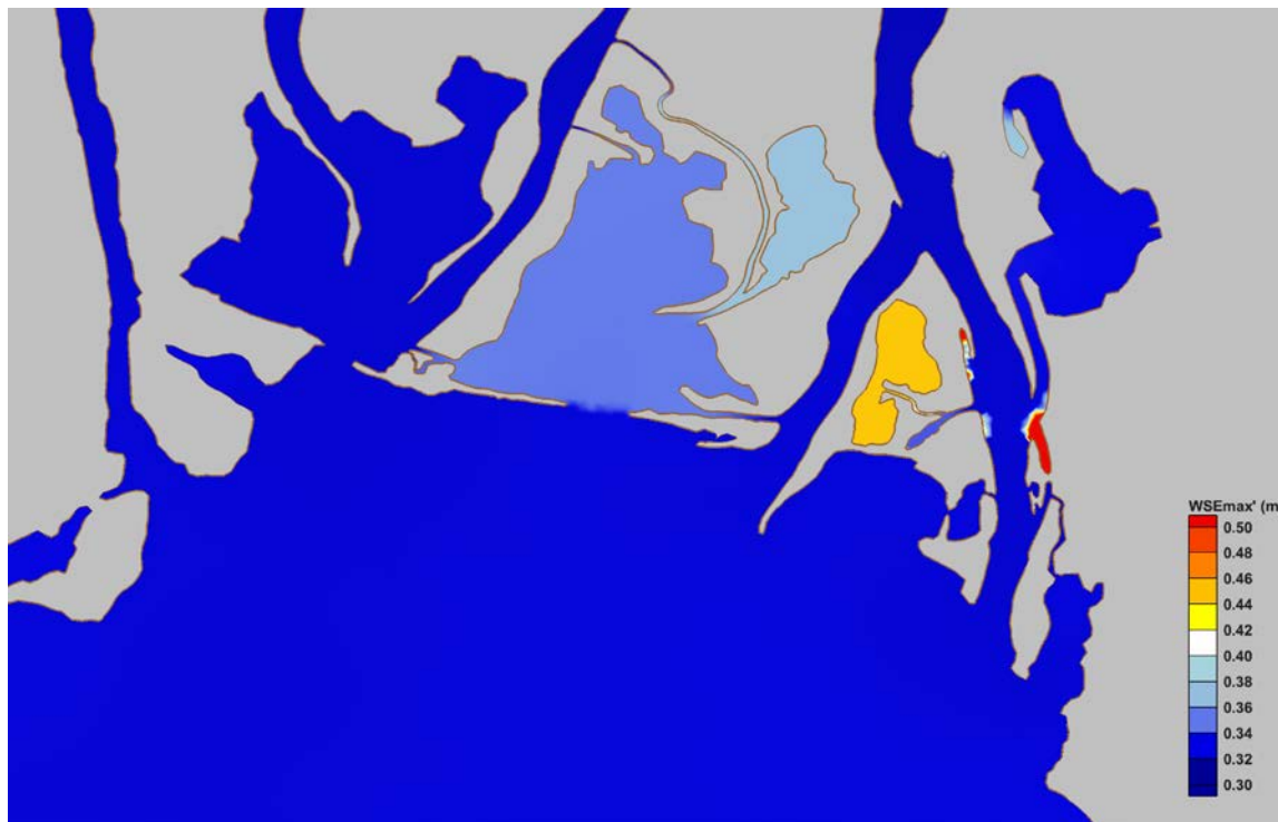
Figure 109. Predicted change in maximum water levels (WSEmax') from Case 002 to Case 112.
