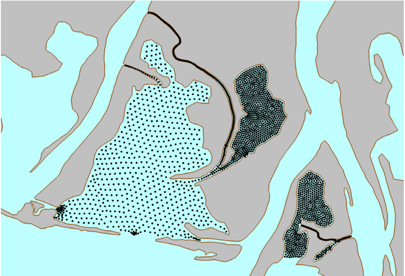
Figure 33. Distribution and initial position of passive particles used in LPTM simulations (black dots). The distribution and initial position of particles was the same for each simulation. The mesh corresponding to Case 412 (all open) is shown for reference.
