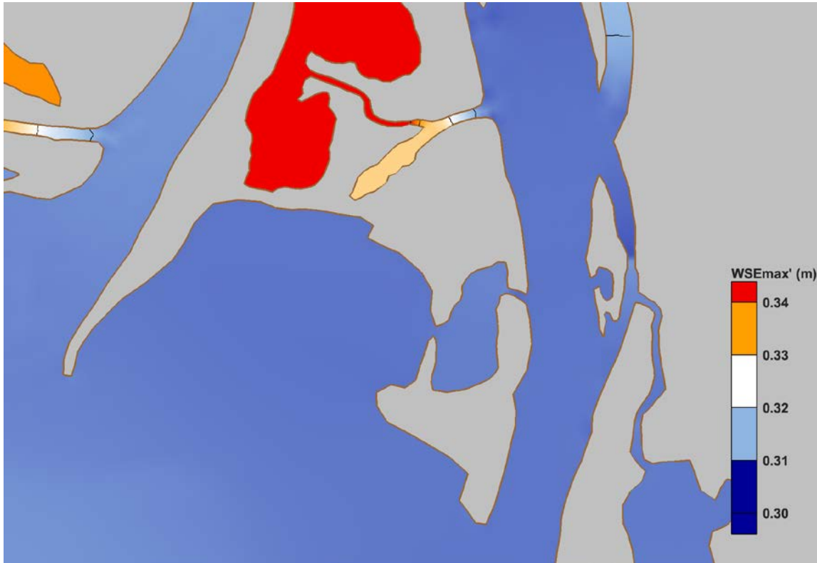
Figure 127. Predicted change in maximum water levels (WSEmax') from Case 002 to Case 312.
