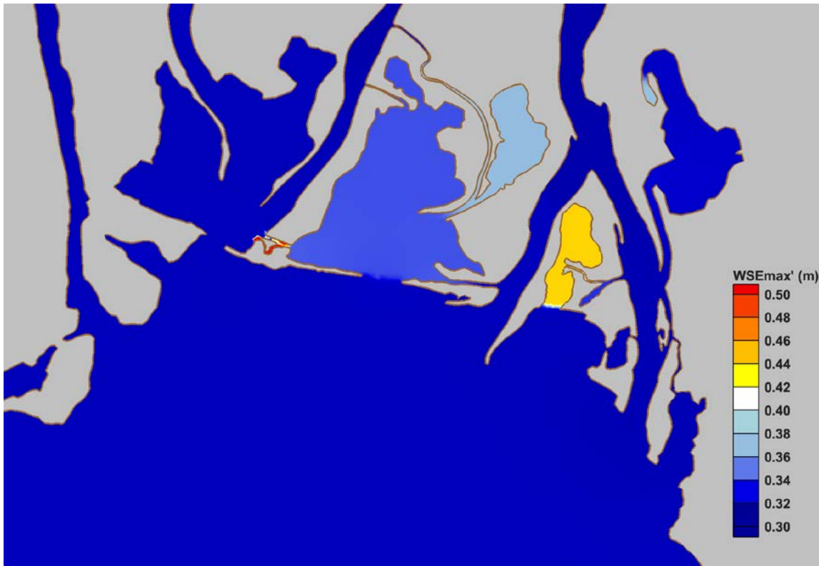
Figure 134. Predicted change in maximum water levels (WSEmax') from Case 002 to Case 412.
