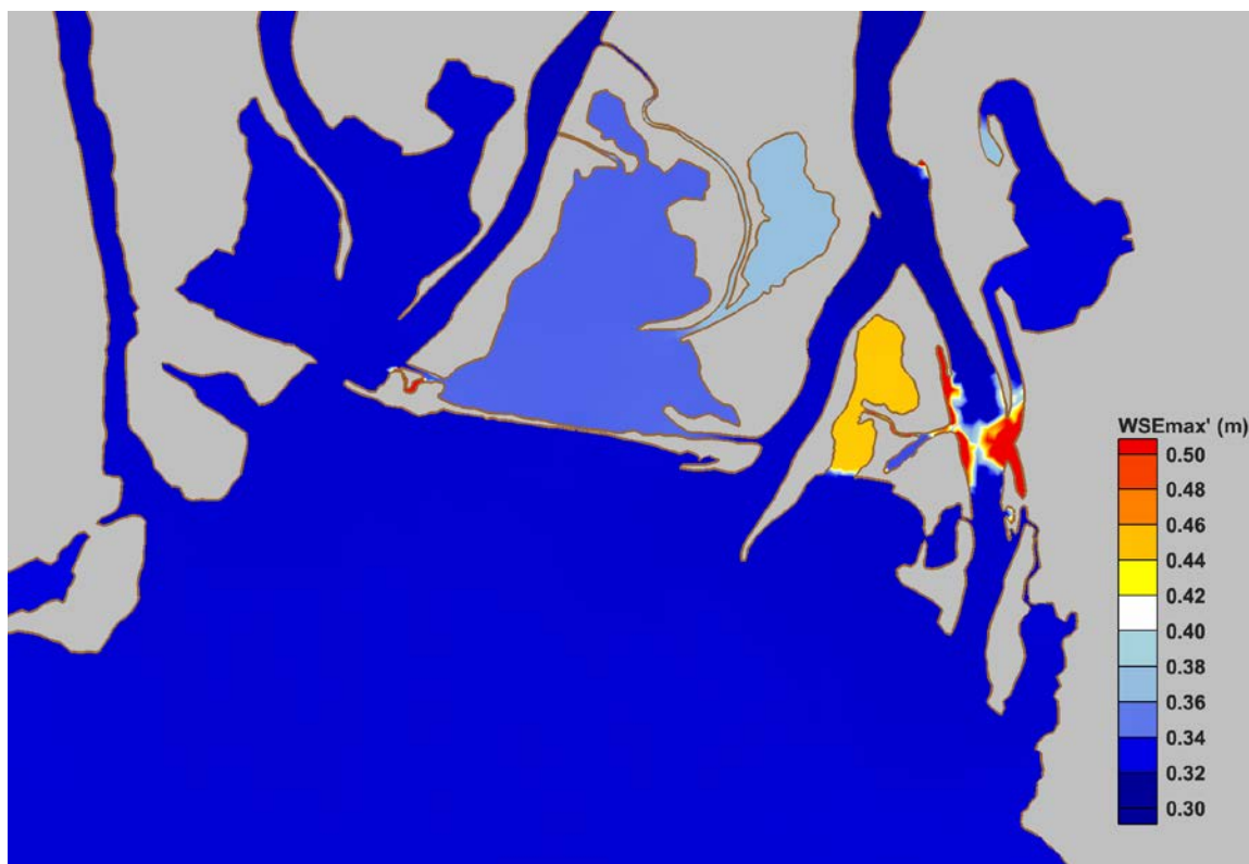
Figure 118. Predicted change in maximum water levels (WSEmax') from Case 002 to Case 212.
