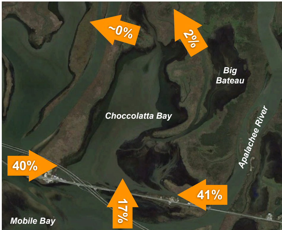
Figure 37. Distribution and direction of tidal exchange volumes for Choccolatta Bay under existing conditions (Case 002). Values are shown as percentages of the total volume of water exchanged.
