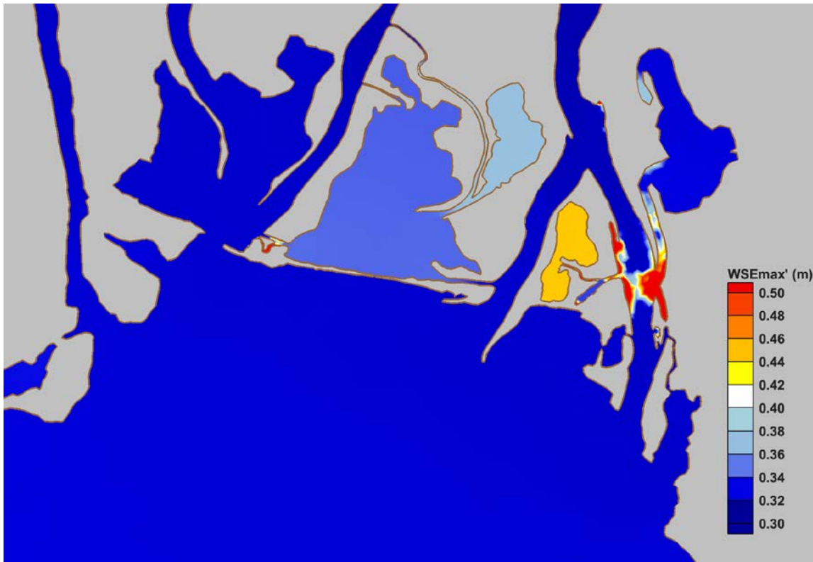
Figure 101. Predicted change in maximum water levels (WSEmax) in the study area from Case 002 to Case 012.
