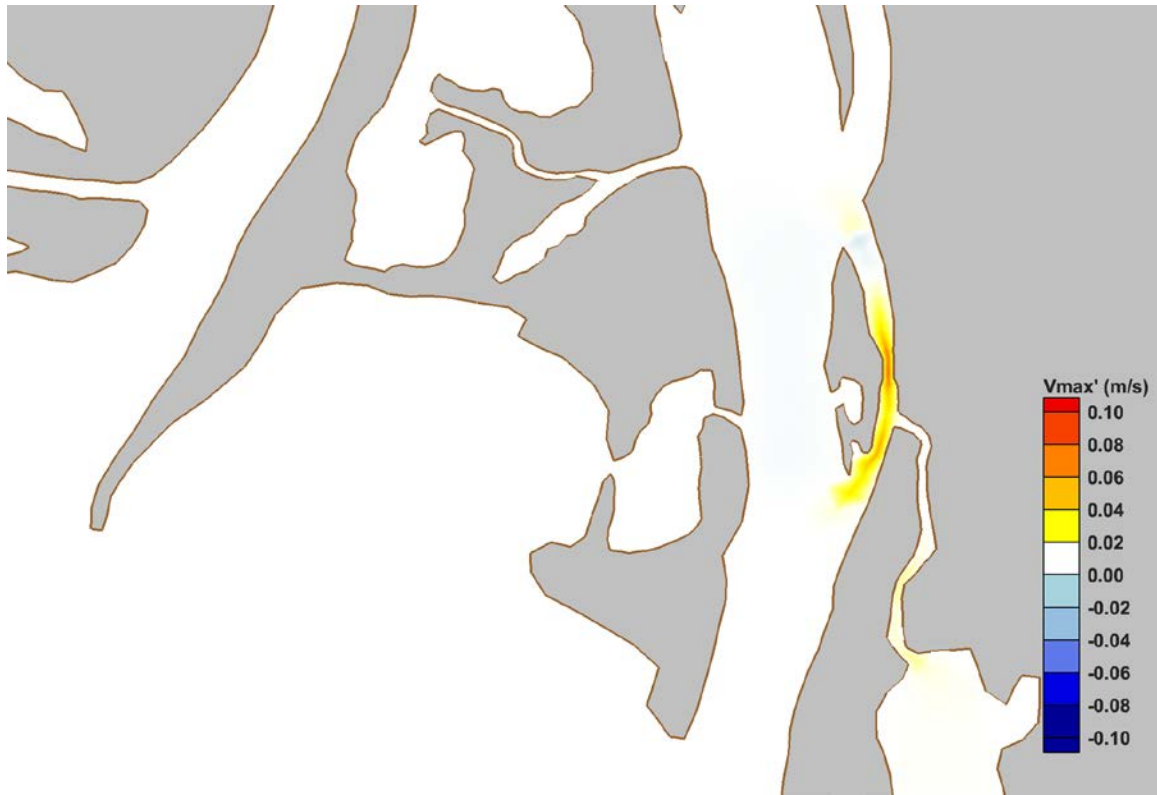
Figure 66. Predicted change in maximum water velocity ( V_{max}' ) from Case 002 to Case 302.
