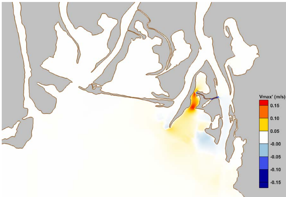
Figure 57. Predicted change in maximum depth-averaged velocity ( V_{\text{max}}' ) between Case 202 and Case 002.
