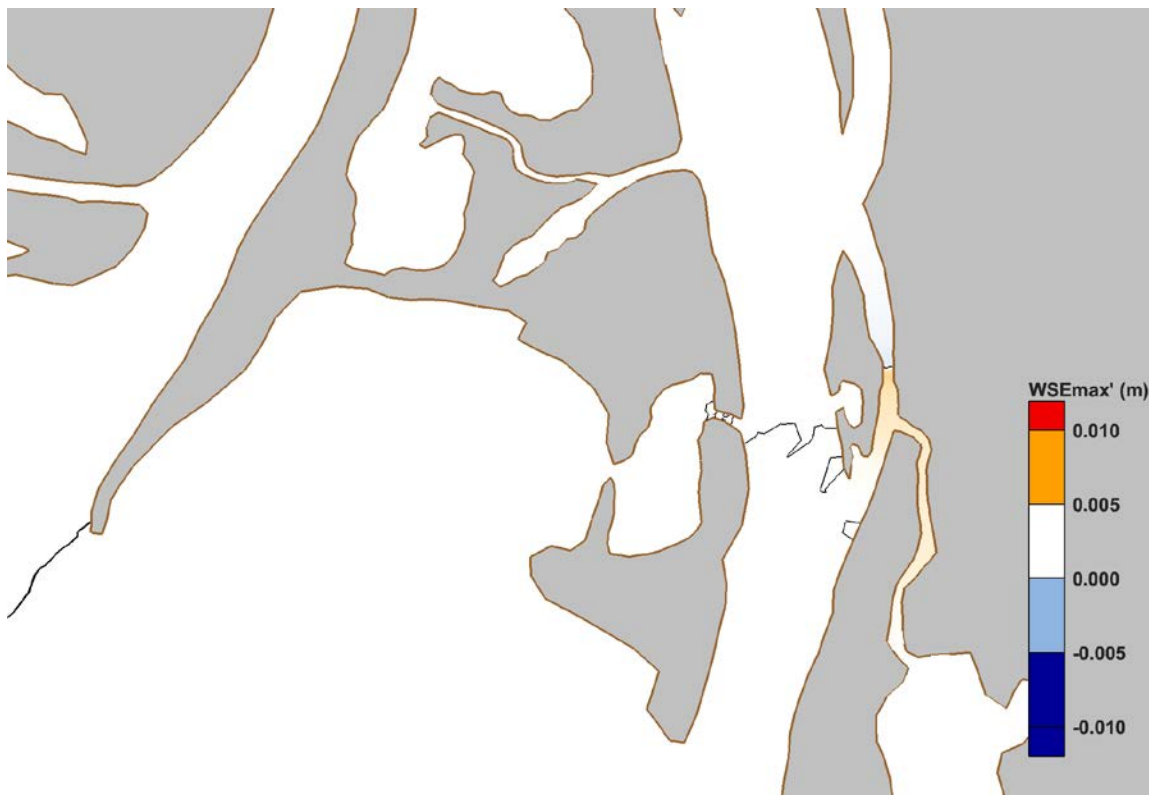
Figure 65. Predicted change in maximum water elevation (WSEmax') from Case 002 to Case 302.
